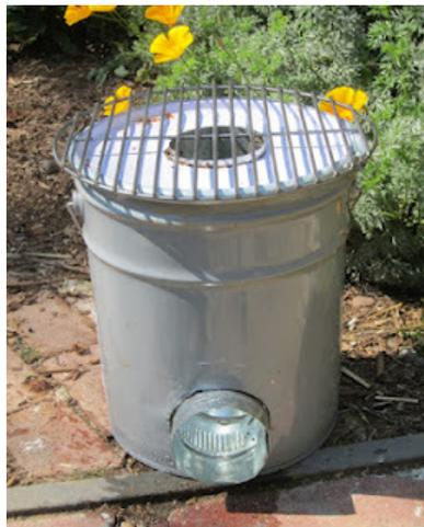
The principle behind a rocket stove is simple--rather than cooking on an open fire, you burn wood in an insulated chimney. Rocket stoves are highly efficient and easy to make. They run on twigs, so you can avoid cutting down a whole tree just to cook dinner.
