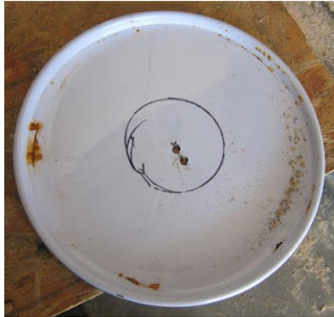
I traced the outline of the vent pipe on to the lid of the bucket and cut this hole out with a jig saw. Tin snips would also have worked.
