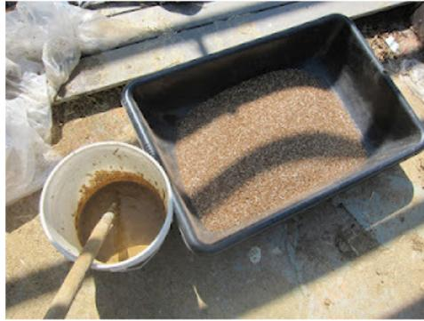
I used one part clay (harvested from the yard) to six parts vermiculite as my insulation material. Mixed with water, the clay holds the vermiculite together. I could also have used dry wood ash, but I had the vermiculite and clay on hand so that's what I went with.
