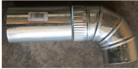
Using a piece of 4" vent pipe and a 90° elbow, I made the chimney. See the pdf for the exact dimensions.
