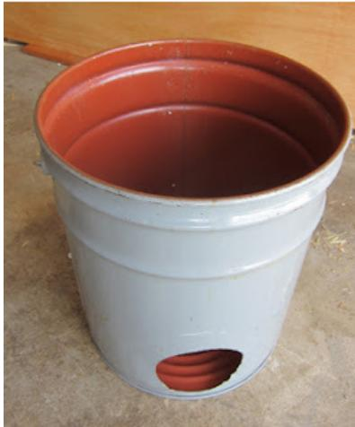
Using the vent pipe as a guide again, I cut out a 4" hole near the bottom of the bucket.
