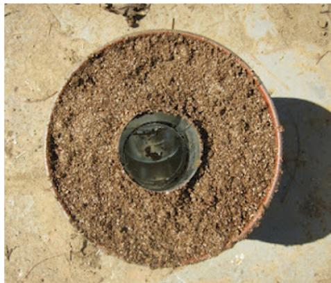
With the vent pipe in place, I packed the insulation into the bucket and let it dry for a few days before putting the lid on.
