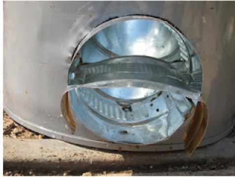
Next you want to get yourself a tin can, take off both ends and open it up with tin snips. Cut a piece to serve as a shelf in the mouth of the pipe. It should be about 4" long--so it sits forward in the mouth of the vent. The rear part of the vent, where the fire burns, is open. The twigs rest on top of the shelf, the lower half is for drawing air.
