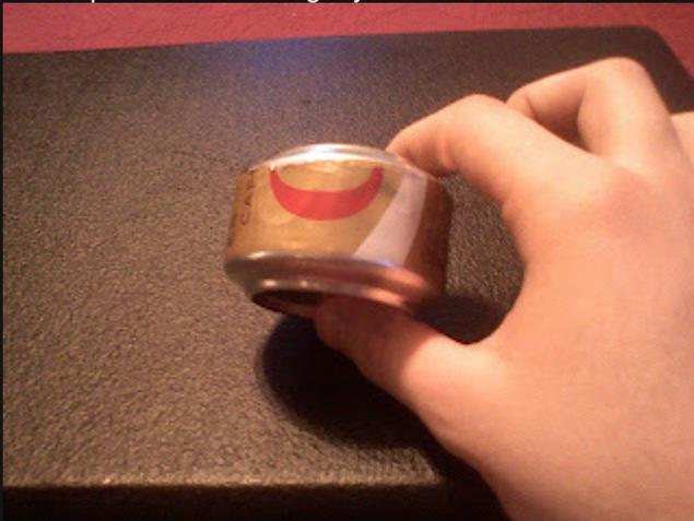
6. Use a thumbtack to place a small hole in the lip of the upper can. The metal is fairly thick at this point, so it might take a little bit of force.
