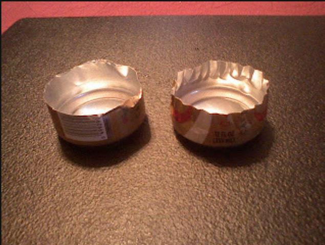
4. On one of the cans, you should crimp the top. Do this by gripping the can with a pair of pliers every half inch and twisting.
